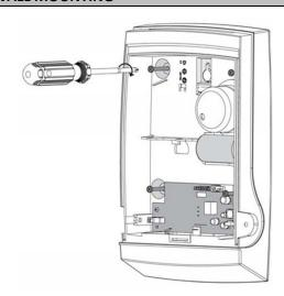
Figure 3 Wall installation
